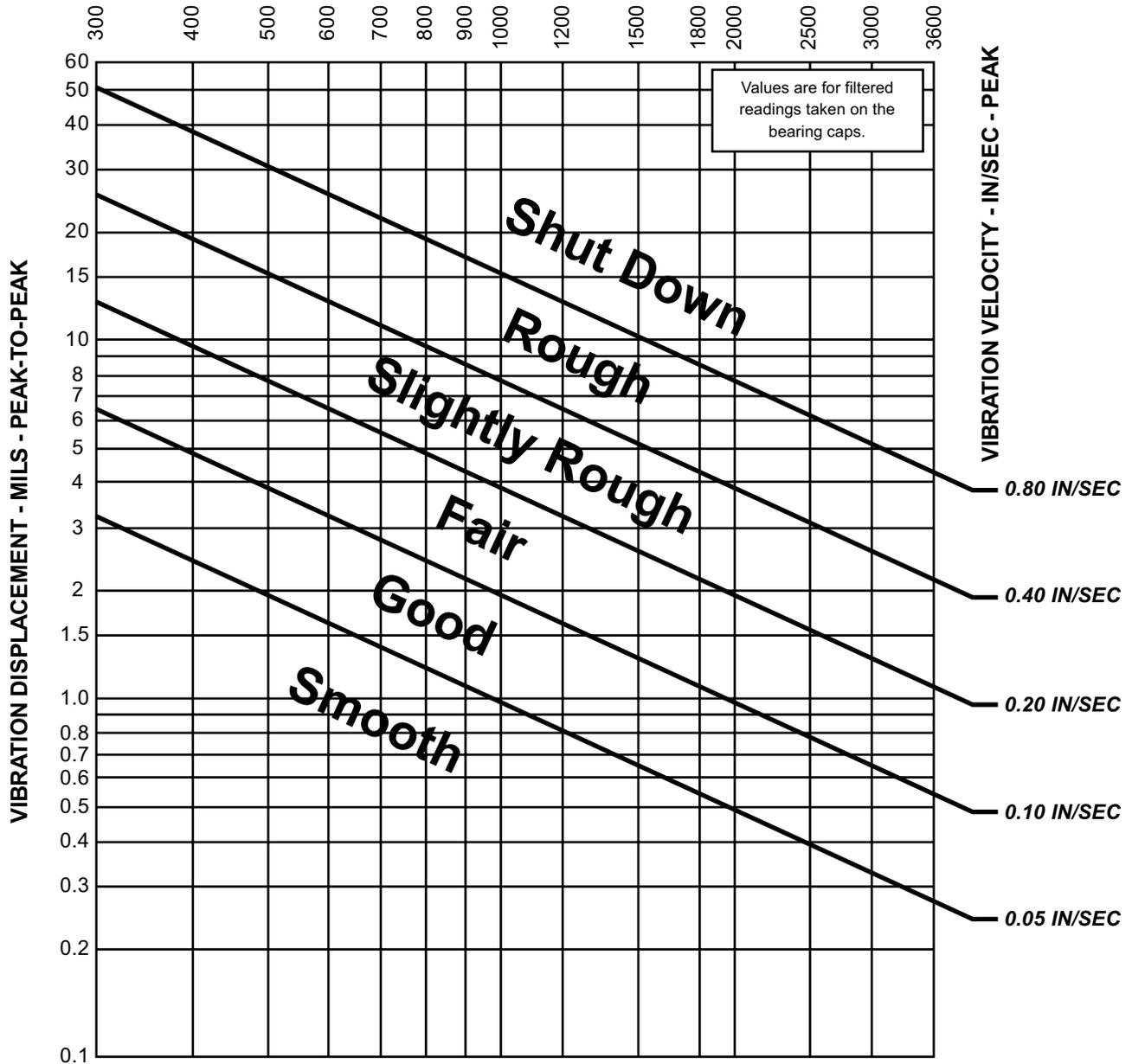
\*Frequency corresponds to RPM when dynamic imbalance is the cause of vibration.
