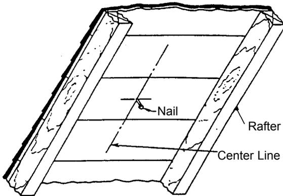
Drive a long nail or drill a pilot hole thru the underside of the roof to center the ventilator between the rafters.
