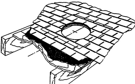
Cut the fan inlet hole thru the roof utilizing the nail or the pilot hole as the center point - use an appropriate cutting tool.
